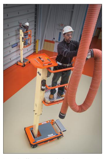
Non-powered **EcoLift**" vertical lifts are an eco-friendly alternative to your powered access needs. They are hydraulic oil and battery free. And with no need to charge the **EcoLift**" Series has no energy consumption.
